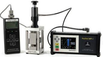
Adhesion testers include everything needed for testing: Adhesion Tester, built-in rechargeable NiMH battery with charger, dollies, abrasive pad, cutting tool, glue with mixing sticks and palettes, cotton swabs, USB cable, PosiSoft Software, instruction booklet, shoulder strap (AT-A only), Certificate of Calibration traceable to NIST, two-year warranty, and sturdy, lightweight carrying case
